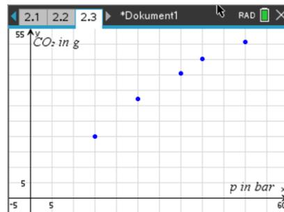
Solubility of carbon dioxide in g per 1 liter of water as a function of pressure at a temperature of  $\vartheta = 20\text{ °C}$ .
