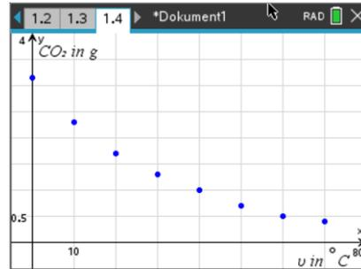
Solubility of carbon dioxide in g per liter of water as a function of temperature at  $p = 1\text{ bar}$
