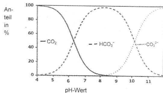
pH dependence of carbon dioxide, hydrogen carbonate and carbonate equilibrium in aqueous solution
